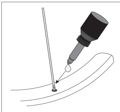
Full stability after 12 hours at room temperature; the wheel can already be used after four hours. The adhesive stays stable at temperatures between -50°C and +150°C.
